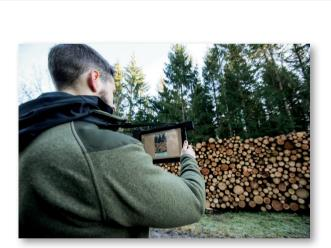
**Measurement of stack:** Now you use the LogStackPro for digital photo measurement of the raw wood stack at the location registered via the LogStackPro app:
